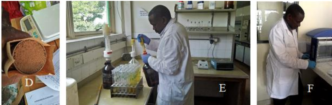
Figure 6. Images Taken During Laboratory Soil Analyses. Photo D: measuring of soil bulk density (core sampler Method), E: Chemical analysis of soil elements and F; Electrophoresis MIDI unit for performing electrophoresis of DNA metagenomics.
